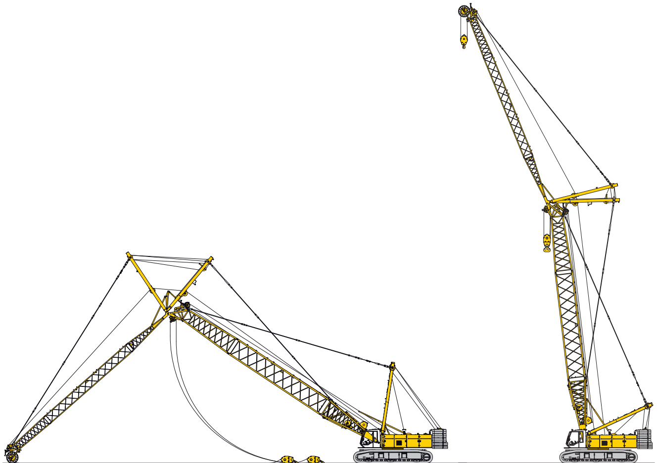
Erecting of main boom and luffing jib
