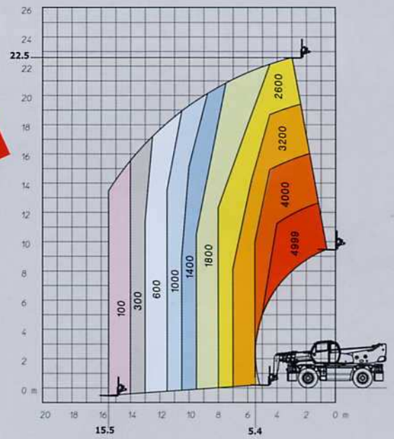
ROTATION ON STABILIZERS FULLY EXTENDED WITH 1000 KG PLATFORM 2,25/4 M
